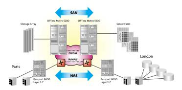
Storage Area Networking solutions use a number of integrated infrastructure components to enable a variety of storage applications. The solutions are typically comprised of a number of disk storage arrays and tape drives connected to a Fibre Channel (FC) switch via FC links. The **OPTera Metro 5200 Multiservice Platform** enables service access delivery providing the solution with flexibility and scalability.
